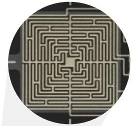
The 4-zone FSR® (Force Sensing Resistor®)
